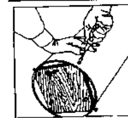
Screwing in the tailgate at all four corners. (Check the fit of the tailgate before installing the mirror).
